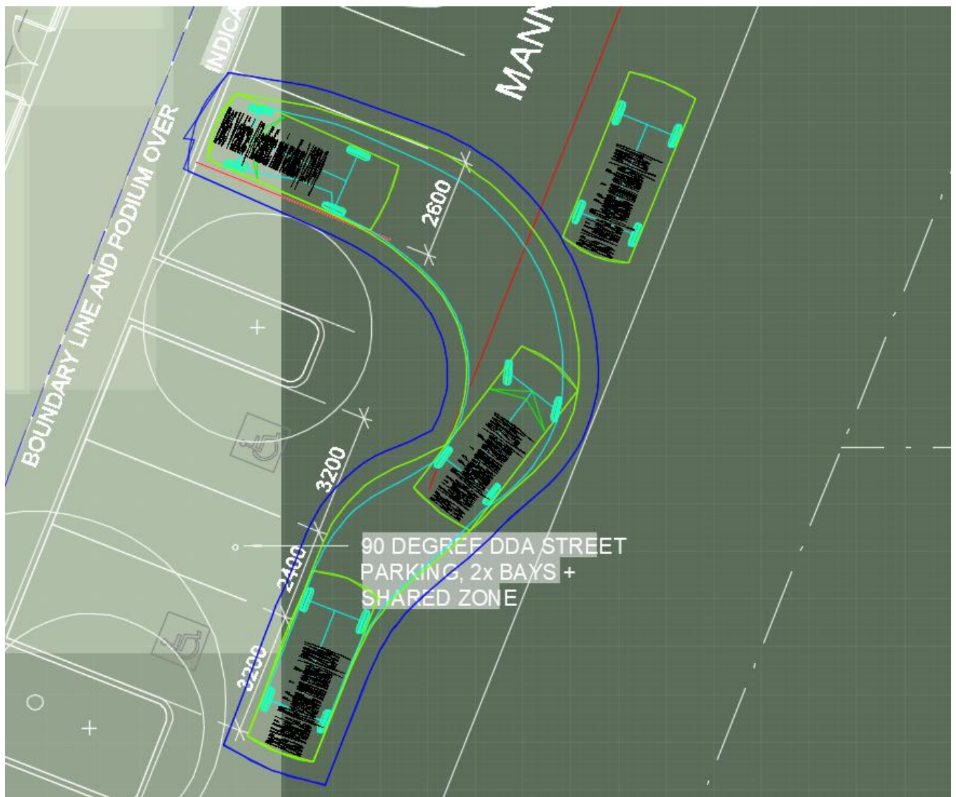
Figure 12: Indicative swept path – vehicle turning left into on-street parking bay
